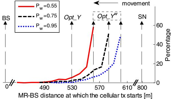
Figure 2. Distribution of the locations at which MR initiates the cellular transmission to the BS ( $\lambda=1/3\text{s}^{-1}$ ) for the ‘Opt-PRBs’ scheme.
